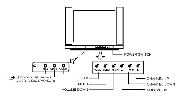
Note: Functions of MENU, TV/AV, ▼VOL ▲, ▼CH ▲ are also provided to the remote controller.
